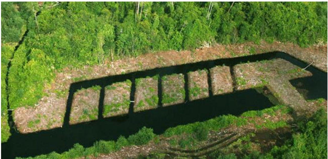
Figure 1. Ecohydrology System with Sisir Pass Design for Peatlands Water Control
